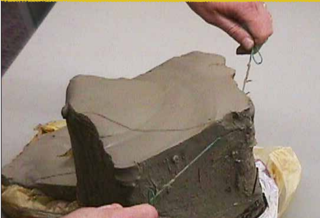
Wire-cutting a slab.
